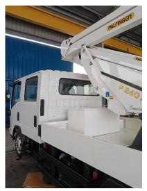
Installation on the ISUZU Double Cabin Truck including fixed sides (0.25m high); floor chequered plate; PTO and as per high quality PALFINGER standards with accessories. Painting: grit blasting SA 2.5 (40microns), primer epoxy-basedcoat, primer filler coat and 2 top coats of WHITE color.
