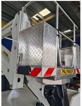
aluminum plate. Below portion of basket is covered by aluminum chequered plate for safety.
